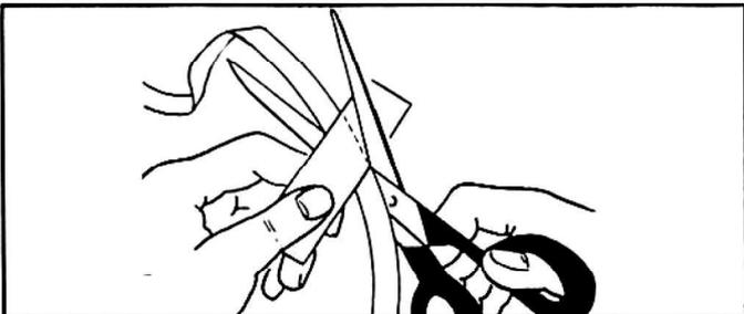
Trim off excess SPLICING TAPE. (Cut into the recording tape backing very slightly as illustrated by dotted lines. This eliminates possibility of a sticky splice.)
