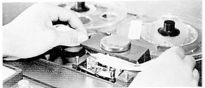
**HEAD DEMAGNETIZATION:** In the course of normal use, the steel pole pieces which form a part of the recording and play back heads become slightly magnetized.
