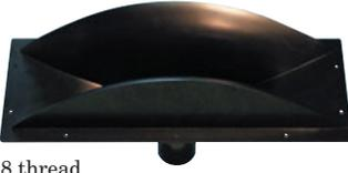
screw-on drivers. Extended lens design delivers outstanding 90° x 40° dispersion and low frequency cutoff of 500Hz. **Specifications:** • Throat diameter: 1" • Front frame dimensions: 16 1/2" x 6 1/4" • Required cutout: 15 1/4" x 4 1/2" • Mounting depth: 5 1/2" • Front extension from baffle: 3 1/4"
